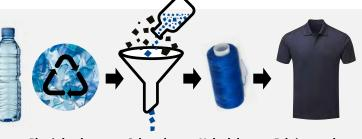
Plastic bottles broken down in to chips Colour dye added
